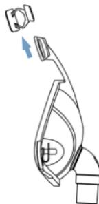
Remove the forehead pad from the installation groove on the mask frame.
