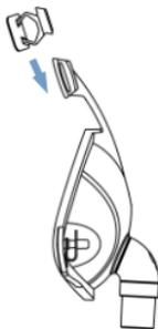
Install the forehead pad onto the upper-half installation groove of the mask frame.
