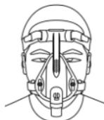
Open the device for the air supply. Attach the respiratory hose with the connector on the base of the mask. Adjust the position of the mask to confirm a tight seal.
