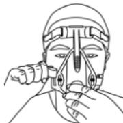
Bring the lower-half straps beneath the ear and encircle the face and then insert it into the fixed hook on the lower-half part of the mask frame.
