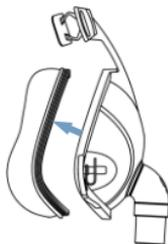
Remove the cushion from the installation groove on the mask frame.
